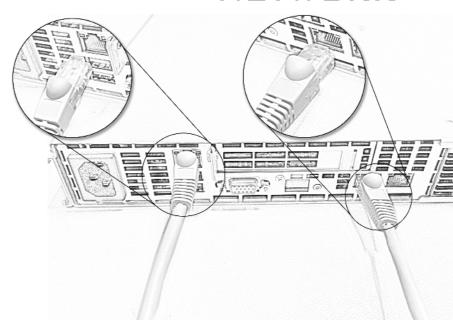
PLUG IN YOUR ETHERNET CABLE TO THE IPMI REMOTE MANAGEMENT PORT. FOR NETWORK ACCESS PLUG A SECOND AVAILABLE NETWORK CABLE INTO ONE OF THE 2X GIGABIT NETWORK PORTS.
