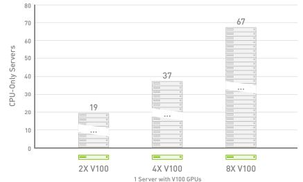
CPU Server: Dual Xeon E5-2690 v4 @ 2.6GHz, GPU Servers: Same as CPU server with NVIDIA® Tesla® V100 for PCIe | NVIDIA CUDA® Version: 9.0.103 | Dataset: 256x256x256 local size | To arrive at CPU node equivalence, we use measured benchmark with up to 8 CPU nodes. Then we use linear scaling to scale beyond 8 nodes.
