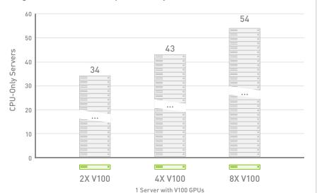
CPU Server: Dual Xeon E5-2690 v4 @ 2.6 GHz, GPU Servers: Same as CPU server with NVIDIA® Tesla® V100 for PCIe | NVIDIA CUDA® Version: 9.0.145 | Dataset: Microsphere | To arrive at CPU node equivalence, we use measured benchmark with up to 8 CPU nodes. Then we use linear scaling to scale beyond 8 nodes.
