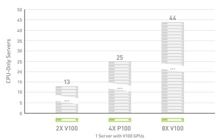
CPU Server: Single Xeon E5-2690 v4 @ 2.6GHz, GPU Servers: Same as CPU server with NVIDIA® Tesla® V100 for PCIe | NVIDIA CUDA® Version: 9.0.103 | Dataset: 350x350x350 | To arrive at CPU node equivalence, we use measured benchmark with up to 8 CPU nodes. Then we use linear scaling to scale beyond 8 nodes.
