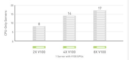
CPU Server: Dual Xeon E5-2690 v4 @ 2.6 GHz, GPU Servers: Same as CPU server with NVIDIA® Tesla® V100 for PCIe | NVIDIA CUDA® Version: 9.0.103 | Dataset: Precision=FP64 | To arrive at CPU node equivalence, we use measured benchmark with up to 8 CPU nodes. Then we use linear scaling to scale beyond 8 nodes.
