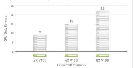
CPU Server: Dual Xeon E5-2690 v4 @ 2.6 GHz, GPU Servers: Same as CPU server with NVIDIA® Tesla® V100 for PCle | NVIDIA CUDA® Version: 9.0.103 | Dataset: A.txt | To arrive at CPU node equivalence, we use measured benchmark with up to 8 CPU nodes. Then we use linear scaling to scale beyond 8 nodes.
