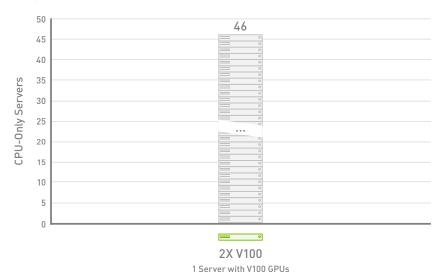
CPU Server: Dual Xeon E5-2690 v4 @ 2.6 GHz, GPU Servers: Same as CPU server with NVIDIA® Tesla® V100 for PCIe | NVIDIA CUDA® Version: 9.0.103 | Dataset: PME-Cellulose\_NVE | To arrive at CPU node equivalence, we use measured benchmark with up to 8 CPU nodes. Then we use linear scaling to scale beyond 8 nodes.
