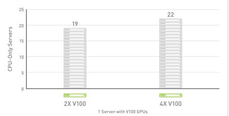
CPU Server: Dual Xeon E5-2690 v4 @ 2.6GHz, GPU Servers: Same as CPU server with NVIDIA® Tesla® V100 for PCIe | NVIDIA CUDA® Version: 9.0.103 | Dataset: bm32 | To arrive at CPU node equivalence, we use measured benchmark with up to 8 CPU nodes. Then we use linear scaling to scale beyond 8 nodes.
