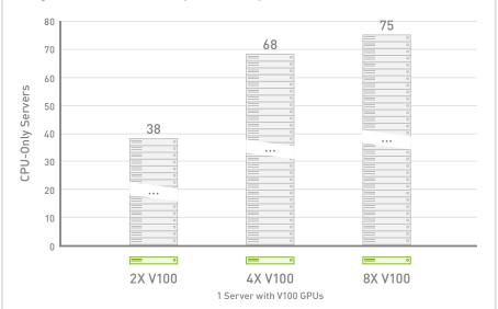
CPU Server: Dual Xeon E5-2690 v4 @ 2.6 GHz, GPU Servers: Same as CPU server with NVIDIA® Tesla® V100 for PCIe | NVIDIA CUDA® Version: 9.0.103 | Dataset: Dslash Wilson-Clove; Precision: Single; Gauge Compression/Recon: 12; Problem Size 32x32x32x64 | To arrive at CPU node equivalence, we use measured benchmark with up to 8 CPU nodes. Then we use linear scaling to scale beyond 8 nodes.
