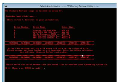
WAIT FOR THE RECOVERY LITH ITY TO LOAD AS SHOWN ABOVE. YOU MAY BE PROMPTED TO PRESS 'ANY KEY TO BOOT FROM USB'. ENTER THE DRIVE NUMBER YOU WISH TO RESTORE TO AND PRESS ENTER.
